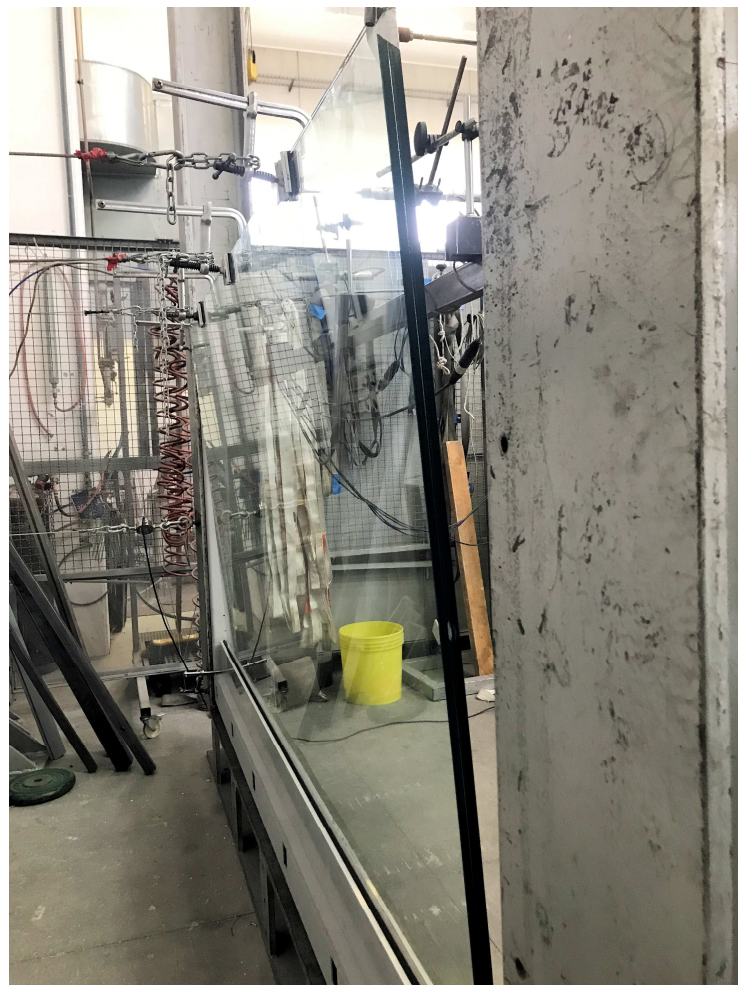
Photograph of the item during resistance to outward horizontal static loading test
